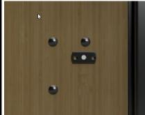
Affix the outside key plate with two #8 self drilling screws. A fillister slotted head screw and toothed lock washer weld nut have been provided for inserting into the outside door keyhole. This screw must be removed for emergency access to the outside keyhole. Life safety codes suggest that no holes are left in a fire door assembly. Holes in listed fire doors must be filled with a steel fastener.
